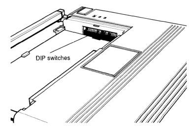
Because the computer is upside down, the DIP switches numbers are upside down and the ON/OFF orientation is reversed. Take care when changing a DIP switch setting that you are changing the correct switch.
